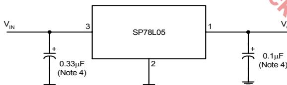
Note 4: Bypass capacitors are recommended for optimum stability and transient response and should be located as close as possible to the regulator.
