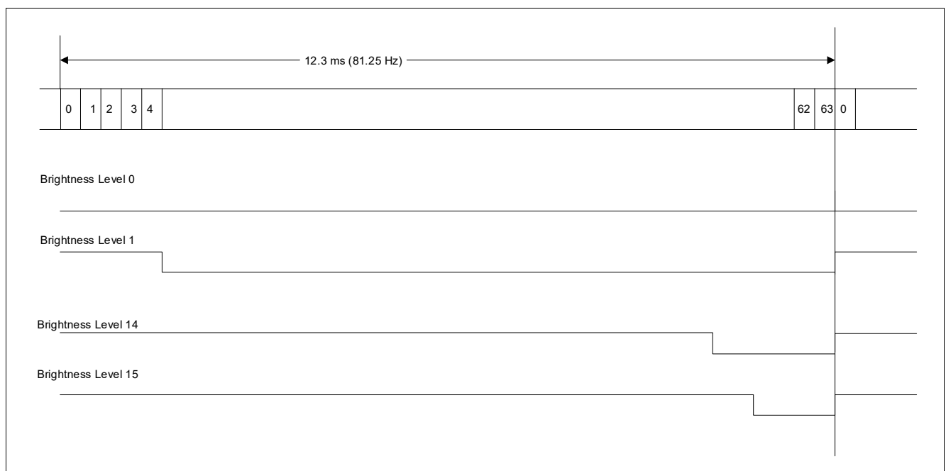
Figure 11 LED Brightness Control By Controlling LED Output Enable/Disable
