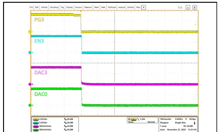
Figure 6: Cold Boot—Fault Response to MxL76500 PG Low
